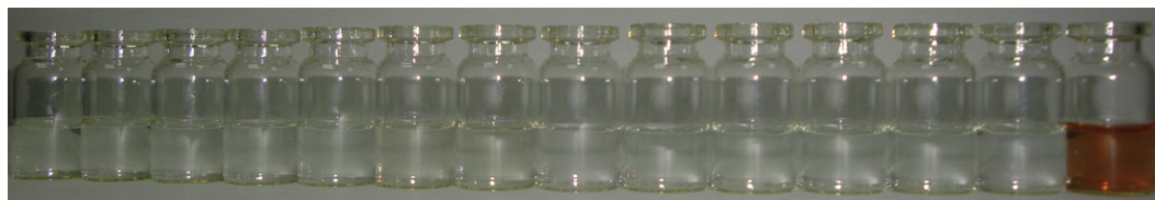
Figure 9. Photograph of the acetonitrile solution of 2d ( 2.0 \times 10^{-5} M) in the presence of different metal ions ( 5 \times 10^{-4} M). The metal ions are None, \text{Ag}^+ , \text{Li}^+ , \text{Ca}^{2+} , \text{Cd}^{2+} , \text{Co}^{2+} , \text{Fe}^{2+} , \text{Hg}^{2+} , \text{Mg}^{2+} , \text{Mn}^{2+} , \text{Ni}^{2+} , \text{Pb}^{2+} , \text{Zn}^{2+} and \text{Cu}^{2+} , respectively, from left to right.
